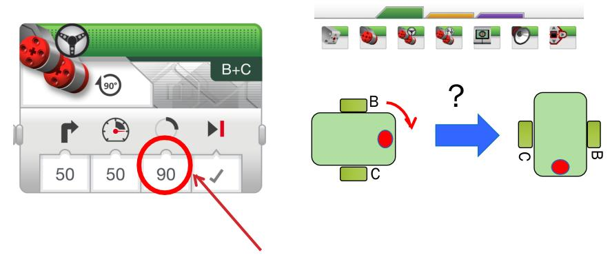
Program your robot to turn 90 degrees....Does the robot actually turn 90 degrees if you just pick 90 degrees for distance?
