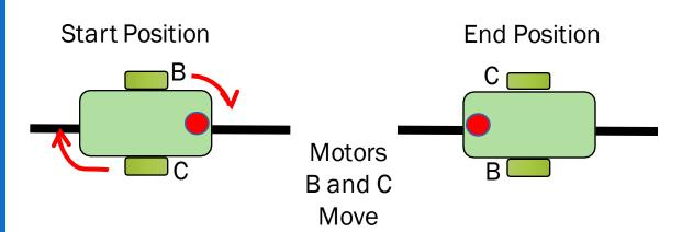
Notice where the robot ends in both pictures after a 180 degree turn.
