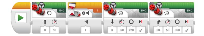
Move forward until touch The touch sensor is set to compare → state → pressed mode.
