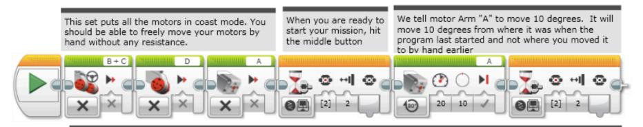
This code shows that the motor arm (A) will not be predictable no matter how much you reset the arm by hand. It's movement is based on where the arm last was. Move the arm by hand at least 90 degrees to see the difference.
