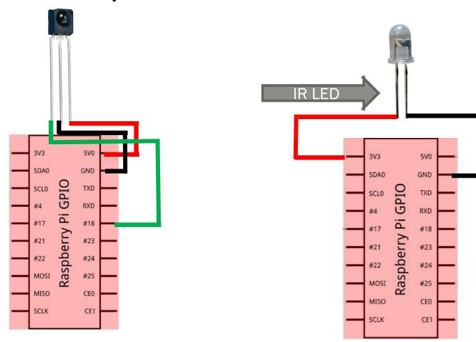
Configuration based on IR sensor available on Adafruit (Product link)
