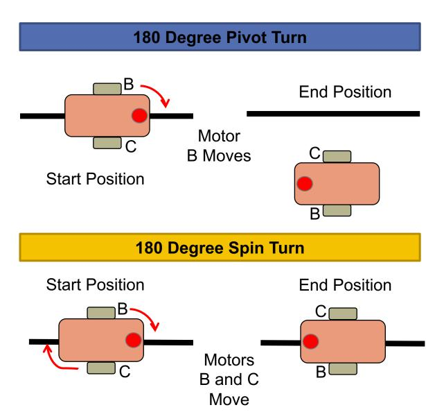
Notice where the robot ends in both pictures after a 180 degree turn.
