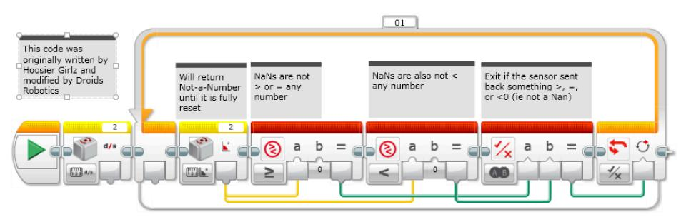
This version of the calibration leaves the gyro in angle mode. This is probably the most common way to use the gyro. This code takes about 0.1sec to run.
