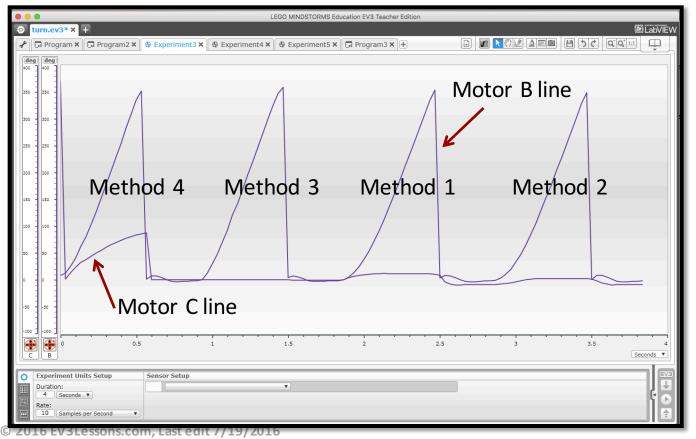
In Method 4, Motor C is dragged along.
